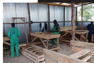
Mud bricks were mainly sourced from the local community, and partly through MoUs with landowners. Timber frames were prepared in workshops within the settlement.
