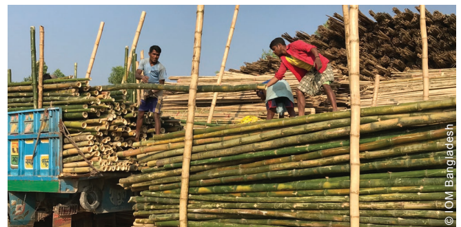
The procurement and logistics for the bamboo required for 100,000 kits needed a large dedicated team and the application of expedited procedures. Because of time constraints, bamboo was untreated and often harvested hurriedly.
