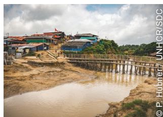
Bridges were erected by refugees and later upgraded to allow better accessibility across the site. Footpaths, stairs and roads all had to be created from scratch.
